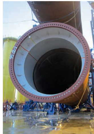
Monopile on deck
