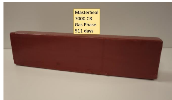
Specimen after 511 days testing and cleaning.
