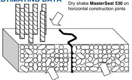
MasterSeal 530 application on vertical construction and day work joints
