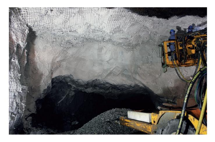
In hard rock mining, oxidation can affect weak strata, causing rock slabbing and roof and wall degradation. Effective surface support and the protection of rock and strata against weathering are critical to the safety and efficiency of any mining operation.
