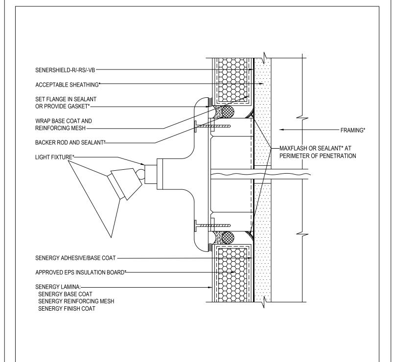
NOTE: DO NOT APPLY FINISH INTO JOINT RECEIVE SEALANT
