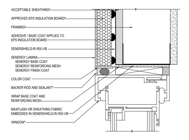
NOTE: DO NOT APPLY FINISH INTO JOINT RECEIVE SEALANT
