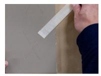
5. Compare the resulting amount of coating that is left intact to the levels included in ASTM D3359 for a rating.
