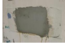
5. Once the test material has cured/dried, take the loose end of mesh or fabric and pull it straight out from the wall surface.
