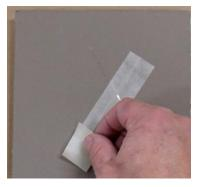
4. The tape is removed by grabbing the free end and pulling it off rapidly back on itself at a 180° angle, or as close to 180° as possible.
