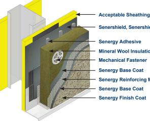
Senershield, Senershield-R/-RS/-VB Senergy Adhesive **Mineral Wool Insulation Mechanical Fastener** Senergy Base Coat Senergy Reinforcing Mesh Senergy Base Coat Senergy Finish Coat
