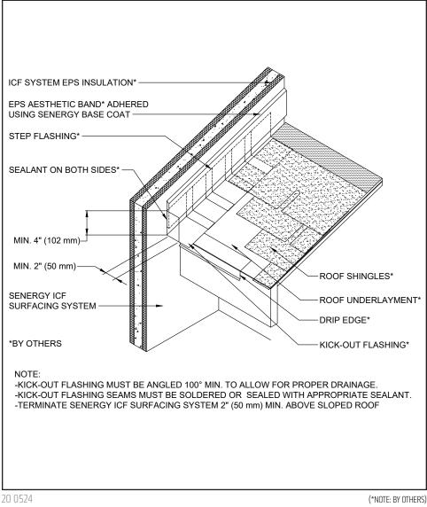
• Terminate system a minimum of 2" (50 mm) above sloped roof.
