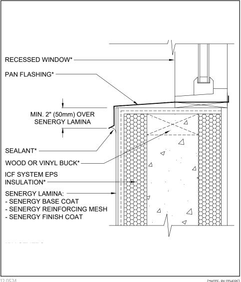
• Ensure that metal pan flashing extends onto the system a minimum of 2" (50 mm) down the face and that end dams are provided.
