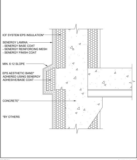
• On horizontal projections greater than 1" (25mm) maintain a minimum 6:12 slope.
