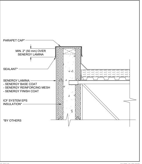
• Ensure that metal coping/flashing extends onto the system a minimum of 2" (50 mm) down the face.
