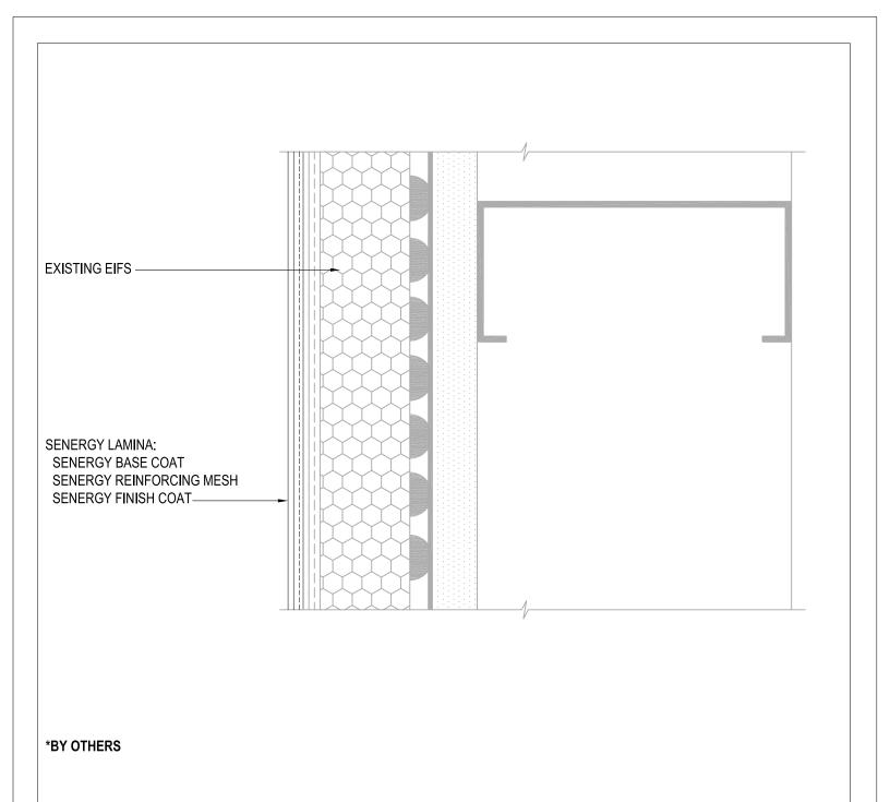
REFERENCE SMART EIFS PROCEDURES AND RESURFACING SPECIFICATION FOR FURTHER INFORMATION
