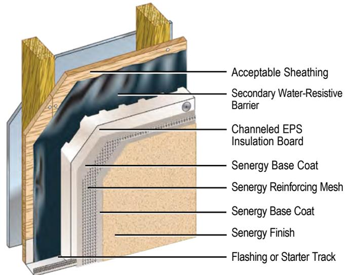
Senturion II is a mechanically attached Class PB EIFS with drainage incorporating a channeled EPS insulation board and a water-resistive barrier.
