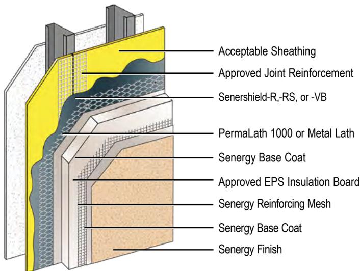
Adhered Mat Design is an EIFS with drainage incorporating an unobstructed drainage plane and an air/water-resistive barrier that provides maximum wind load resistance.
