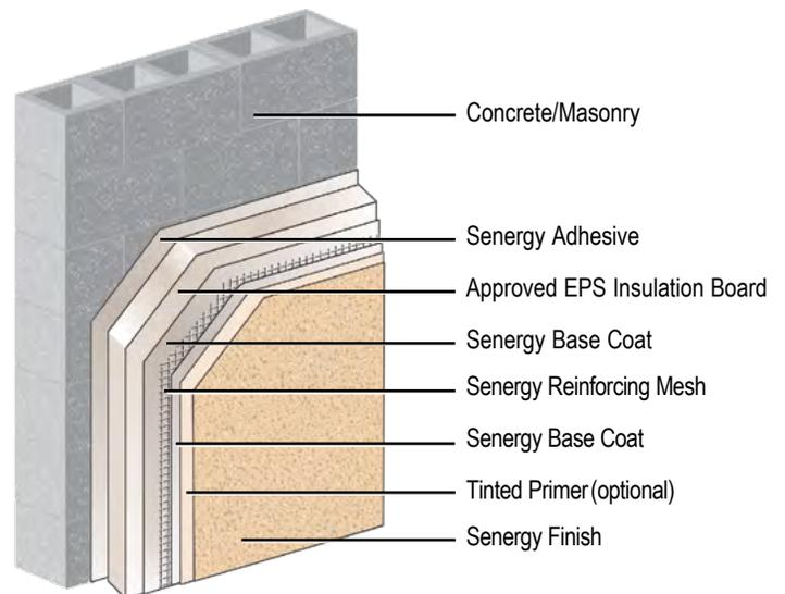
Senerflex Classic PB is a mechanically and/or adhesively attached, non-drainage Class PB EIFS which provides primary barrier moisture control.
