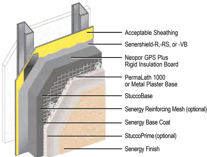
Senergy Platinum CI Stucco Plus is a premium continuously insulated cement plaster/stucco featuring Neopor GPS Plus Rigid Insulation Board and a fluid-applied air/water-resistive barrier.
