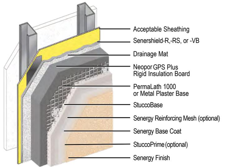
Senergy Platinum CI Stucco Ultra is a premium continuously insulated cement plaster/stucco rain screen system with enhanced water management featuring Neopor GPS Plus Rigid Insulation Board.
