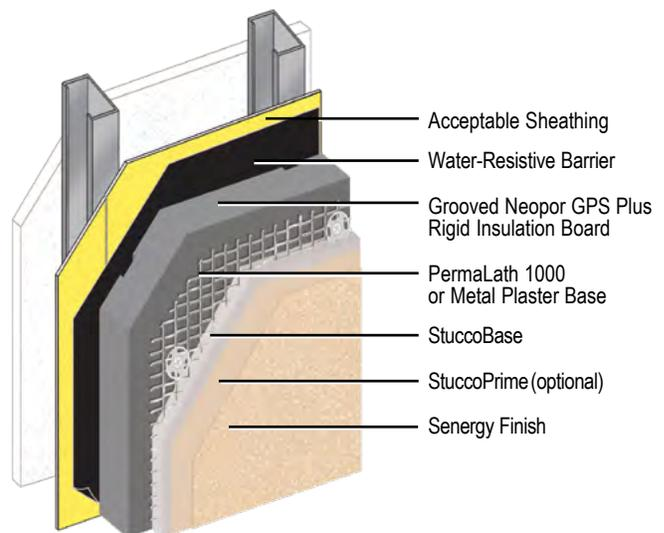
Senergy Platinum CI Stucco is a continuously insulated cement plaster/stucco system featuring Neopor GPS Plus Rigid Insulation Board.
