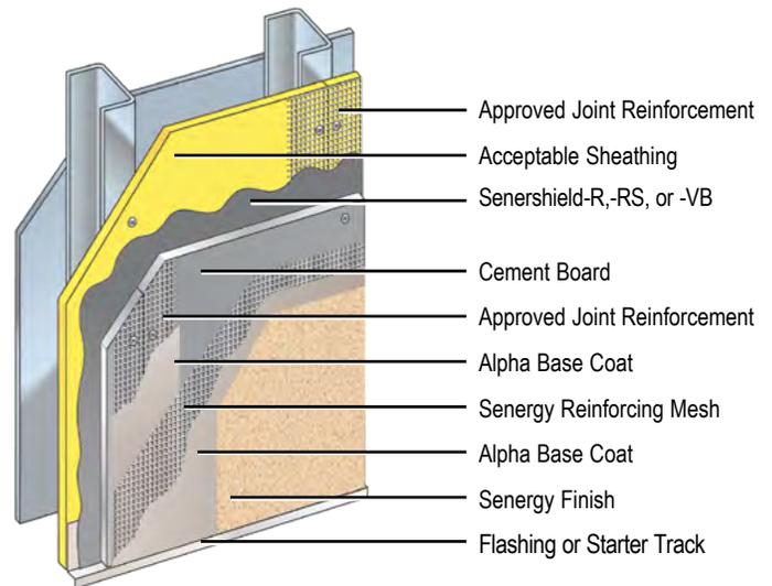
Cement-Board Stucco 1000 is a highly impact and puncture resistant wall system with the look of stucco.
