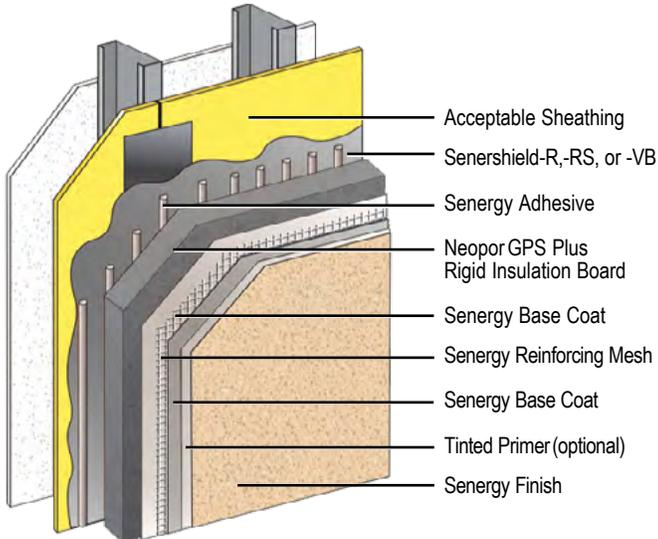
Senergy Platinum CI (Continuous Insulation) is an exterior cladding system featuring Neopor® advanced insulation technology.
