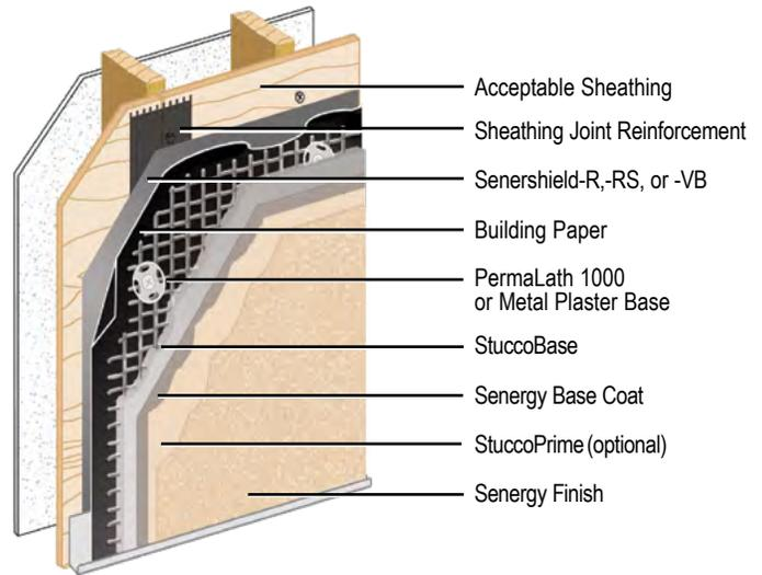
Sentry Stucco Plus is a highly advanced Portland cement-based exterior wall system. It features a fluid-applied air/water-resistant barrier, available rustproof fiberglass lath, a base coat and textured finishes.
