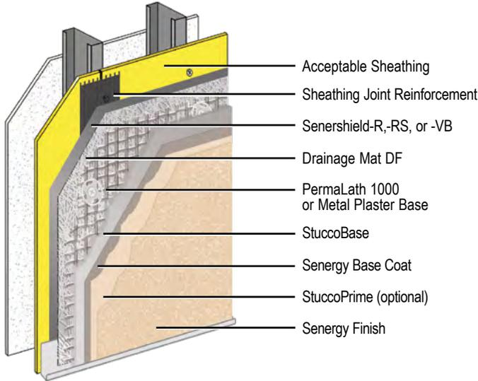
Sentry Stucco Ultra is a highly advanced Portland cement-based exterior wall system. Its features a rainscreen design for maximum water management security, a fluid-applied air/water-resistant barrier, drainage mat, available rustproof fiberglass lath, a base coat and textured finishes.
