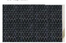
Cut the dry fiber fabric into the proper width and length using shears or a utility knife.
