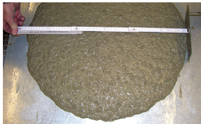
Sprayed concrete quality testing
