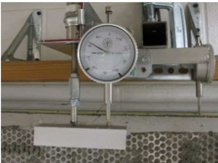
Figure 5 Dial Gauges to Measure Deflections
