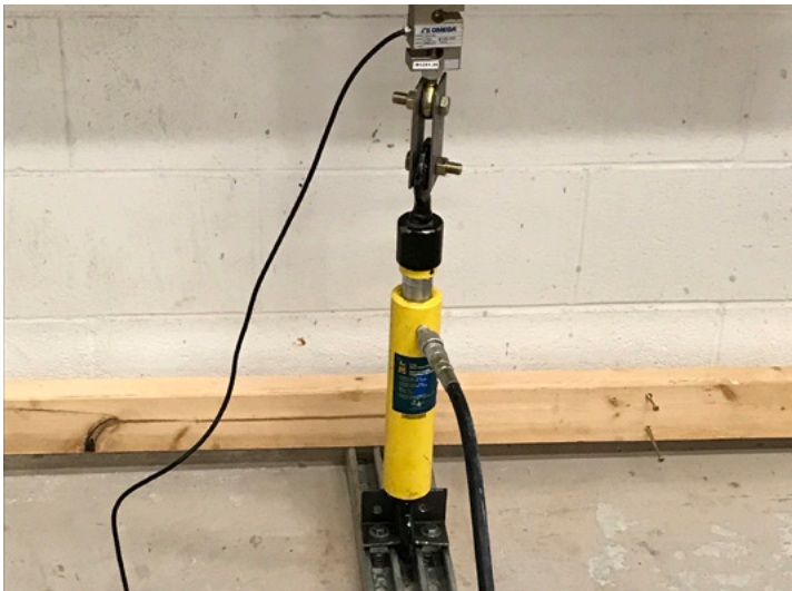
Figure 4 Hydraulic Ram with Load Cell at Base of Test Specimen
