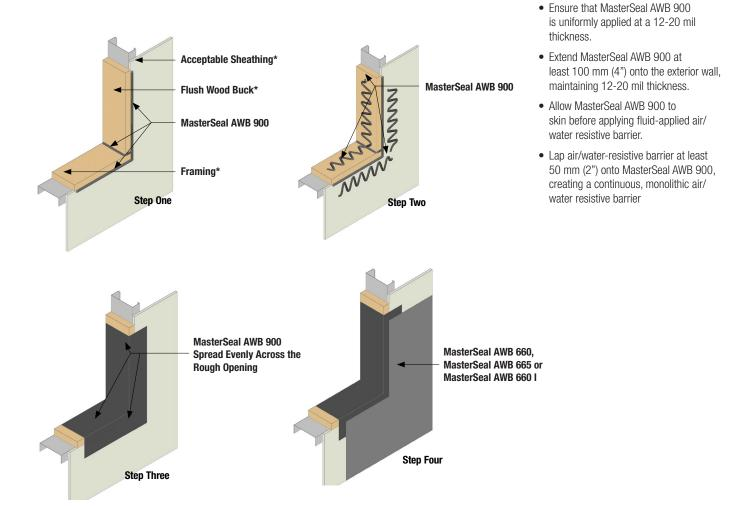
TYPICAL ROUGH OPENING TREATMENT WITH MASTERSEAL AWB 900 ON MASONRY OR CONCRETE CONSTRUCTION WITH A RECESSED BUCK
