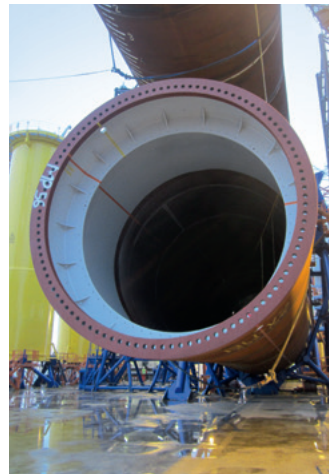
Monopile on deck
