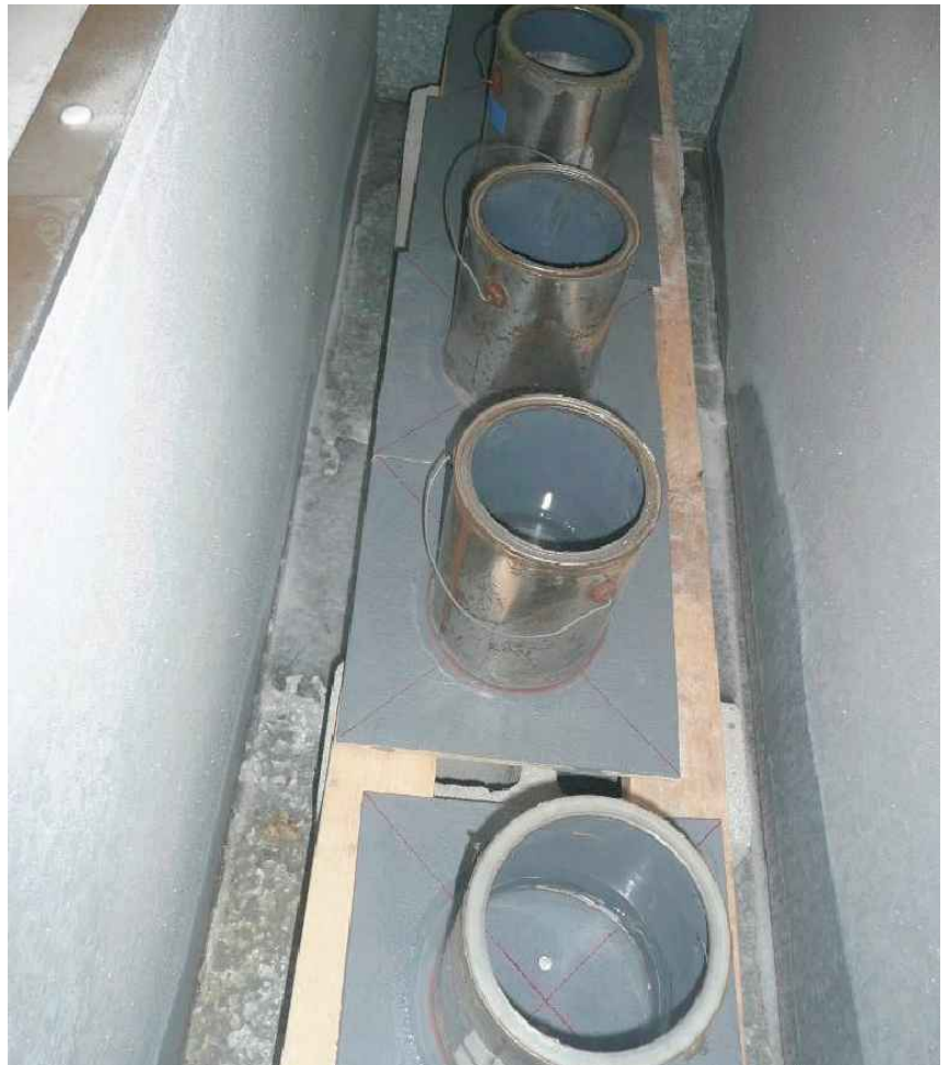
ASTM D1970 test apparatus. This test measures the ability of a barrier material to self-seal around two nails in a manner sufficient to prevent a column of water from seeping through the penetration.
