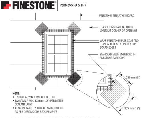
PD-05 TYPICAL INSULATION BOARDS/REINFORCING MESH APPLICATION AT OPENINGS
