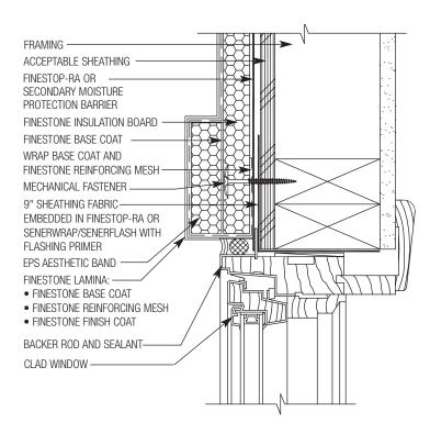
PD-06 TYPICAL CLAD WINDOW JAMB WITH AESTHETIC BAND
