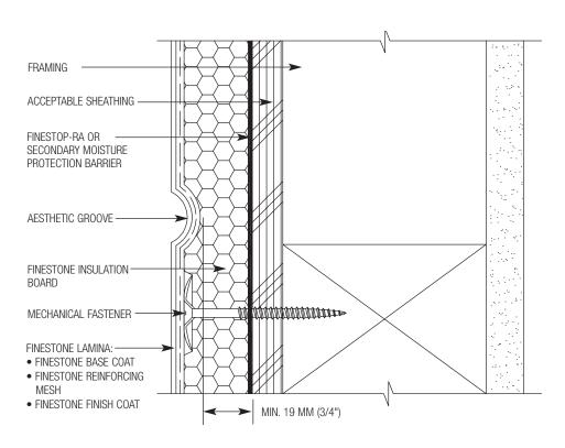
PD-04 TYPICAL AESTHETIC GROOVE (PLAN VIEW)
