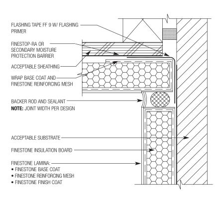
PD-16 TYPICAL EXPANSION JOINT AT CHANGE IN SUBSTRATE (PLAN VIEW)
