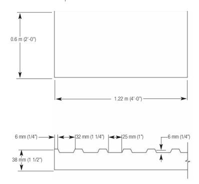
PD-29 TYPICAL PEBBLETEX-D7 SYSTEM CHANNELED INSULATION BOARD PROFILE
