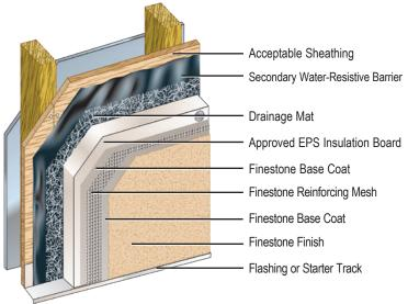
Pebbletex D10 is a mechanically attached Class PB EIFS with drainage incorporating a pre-formed drainage mat and a water-resistive barrier to provide an unobstructed drainage plane.
