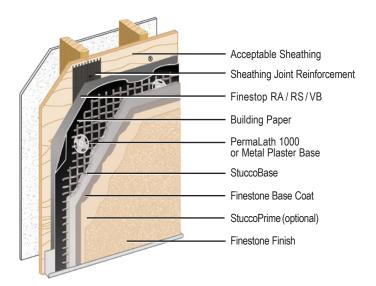
Finestone Stucco Plus is a highly advanced Portland cementbased exterior wall system. It features a fluid-applied air/waterresistive barrier, available rustproof fiberglass lath, a base coat and textured finishes.
