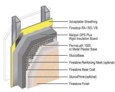
Finestone Platinum CI Stucco Plus is a premium continuously insulated cement plaster/stucco featuring Neopor GPS Plus Rigid Insulation Board and a fluid-applied air/water-resistive barrier.
