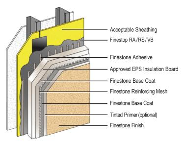
Pebbletex DCA is an adhesively attached, continuously insulated water-drainage exterior cladding incorporating vertical drainage channels and a secondary air/water-resistive barrier.
