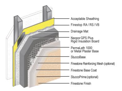
Finestone Platinum CI Stucco Ultra is a premium continuously insulated cement plaster/stucco rain screen system with enhanced water management featuring Neopor GPS Plus Rigid Insulation Board.
