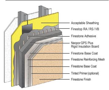
Finestone Platinum CI (Continuous Insulation) is an exterior cladding system featuring Neopor® advanced insulation technology.
