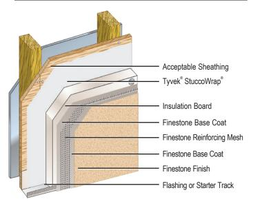
Pebbletex I is a mechanically attached Class PB EIFS with drainage incorporating Tyvek StuccoWrap water-resistive barrier.
