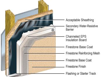
Pebbletex D7 is a mechanically attached Class PB EIFS with drainage incorporating a channeled EPS insulation board and a water-resistive barrier.
