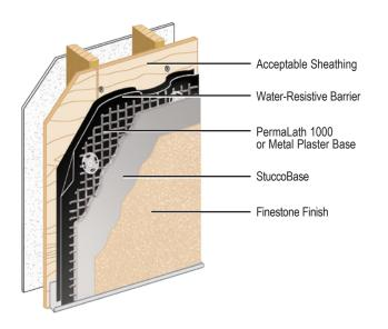
Finestone Stucco Wall System is a Portland cement-based exterior wall system.
