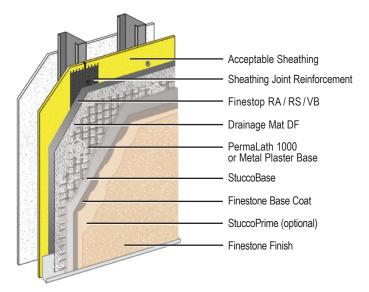
Finestone Stucco Ultra is a highly advanced Portland cementbased exterior wall system. Its features a rainscreen design for maximum water management security, a fluid-applied air/waterresistive barrier, drainage mat, available rustproof fiberglass lath, a base coat and textured finishes.
