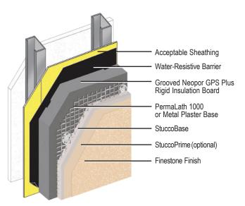
Finestone Platinum CI Stucco is a continuously insulated cement plaster/stucco system featuring Neopor GPS Plus Rigid Insulation Board.
