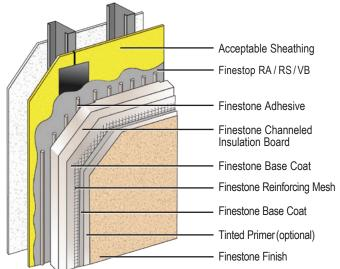
DCA with Channeled Insulation is an adhesively attached, continuously insulated water-drainage exterior cladding incorporating channeled EPS insulation boards and a secondary air/water-resistive barrier for added water management security.
