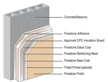
Classic PB is a mechanically and/or adhesively attached, nondrainage Class PB EIFS which provides primary barrier moisture control.
