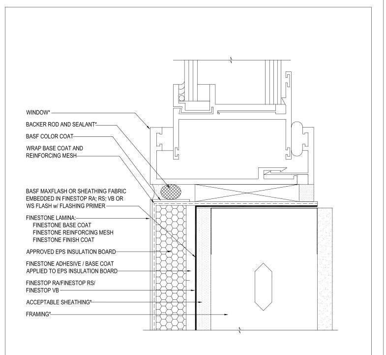
NOTE: DO NOT APPLY FINISH INTO JOINT TO RECEIVE SEALANT
