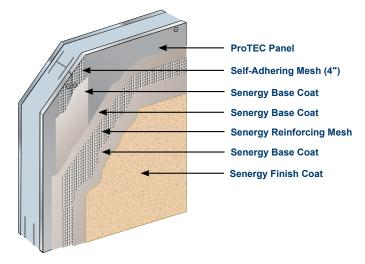
**C.** Apply mixed Base Coat to entire surface of Self-Adhering Mesh Tape (4").
