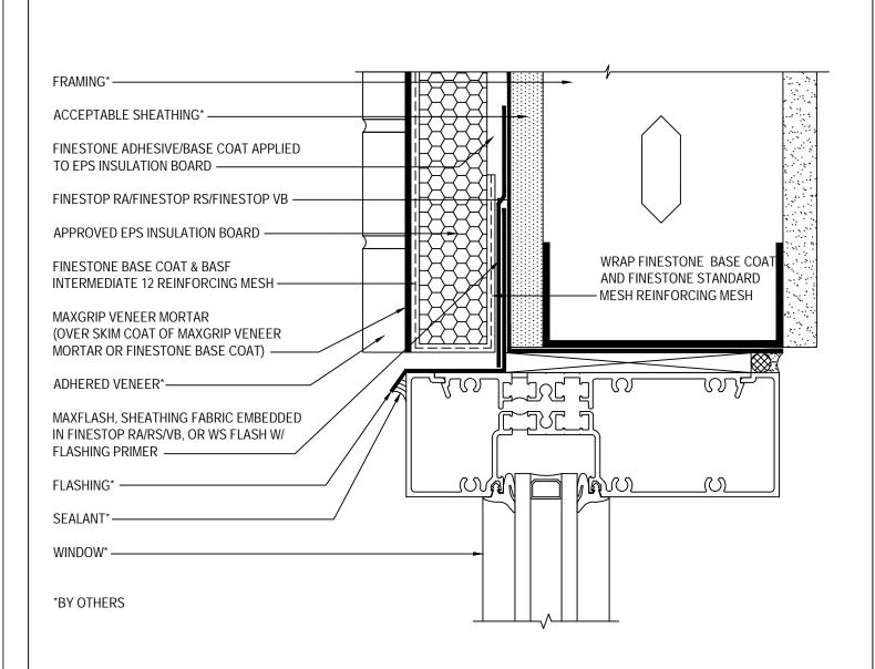
NOTE: WRAP MAXFLASH, SHEATHING FABRIC EMBEDDED IN FINESTOP RA/RS/VB OR WS FLASH W/ FLASHING PRIMER INTO ROUGH OPENING ON HEAD IF INTENDED TO BE AN AIR BARRIER.
