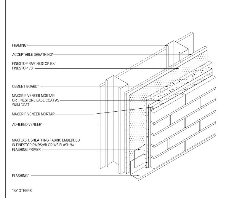
NOTE: Cement board joints are treated with Finestone reinforcing mesh and base coat prior to skim coat application per Finescreen 1000 with MaxGrip Veneer Mortar instructions
