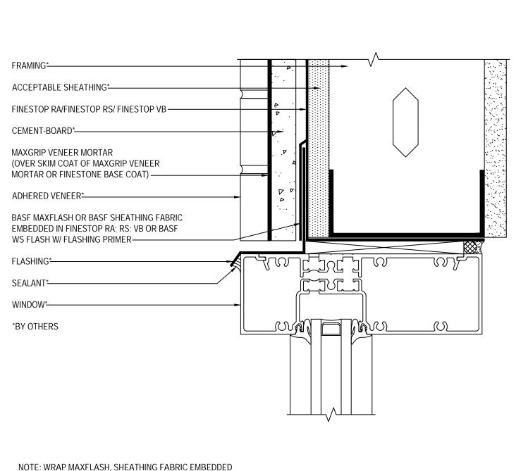
NOTE: WRAP MAXFLASH, SHEATHING FABRIC EMBEDDED IN FINESTOP RA; RS; VB OR WS FLASH W/ FLASHING PRIMER INTO ROUGH OPENING ON HEAD IF ALSO INTENDED TO BE AN AIR BARRIER.
