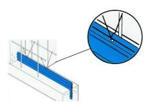
MasterSeal 940 ECJ & EEJ profiles when used on ground slab blinding concrete where a permanent, firm and stable support is given usually require no fixing. The profile is simply laid centrally over the line of the joint to be formed. Fixing to vertical shuttering is simplified by nailing with double headed nails through the outer reinforced flange to provide a firm fixing as shown below.
