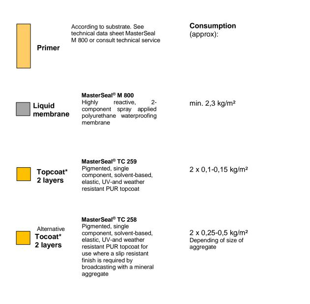
**Hinweis:** Consumptions are indicative and may be higher, depending on substrate roughness, temperature and porosity, as well as waste produced during application.
