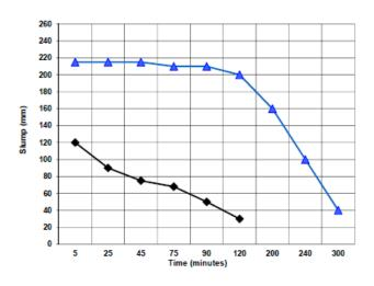
concrete with MasterRheobuild 561: 0.85L/100kg; slump=220mm; w/c=0.47
