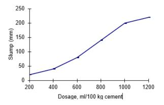
Max size of aggregates - 20 mm Cementitious content - 350 kg/m<sup>3</sup> Temperature 23<sup>o</sup>C.
