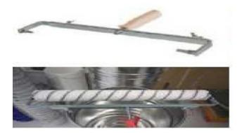
Note: Before starting the application, clean the roll thoroughly with scotch tape to avoid shedding. Ensure full saturation of the roller to avoid uneven coverage. The roller should be double armed to ensure even pressure.
