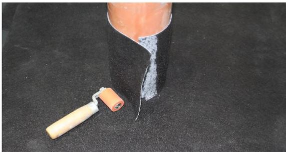
Pipe wrapped with Repair tape
