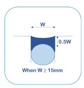
Joint depth is controlled by the use of closed cell backer rod. This also prevents 3-sided adhesion which would be highly detrimental to long term performance of the joint sealant
