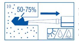
10. Insert the mixing nozzle to the bottom of the hole. Extrude the resin and slowly withdraw the nozzle from the hole. Ensure no air voids are created as the nozzle is withdrawn. Inject resin until the hole is approximately <sup>3</sup>/<sub>4</sub> full and remove the nozzle from the hole. Release the pressure on the cartridge to prevent any further material being extruded accidentally.
