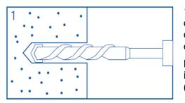
1. Using the SDS Hammer Drill in rotary hammer mode for drilling, with a carbide tipped drill bit of the appropriate size, drill the hole to the required diameter and depth as indicated on the latest **MasterFlow 918 AN** technical data sheet.
