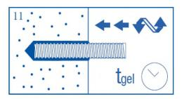
11. Immediately insert the threaded steel anchor element into the hole using a back and forth twisting motion to ensure complete cover, until it reaches the bottom of the hole. Excess resin will be expelled from the hole evenly around the steel element and there shall be no gaps between the anchor element and the wall of the drilled hole.
