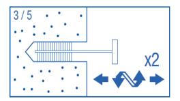
3. Select the correct size Hole Cleaning Brush. Ensure that the brush is in good condition and the correct diameter. Insert the brush to the bottom of hole, using a brush extension if needed to reach the bottom of the hole and withdraw with a twisting motion. There should be positive interaction between the steel bristles of the brush and the sides of the drilled hole.
