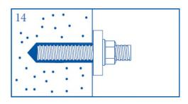
14. Position the fixture and tighten the anchor to the appropriate installation torque. Always allow sufficient curing time BEFORE tightening the anchors.
