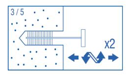
3. Select the correct size Hole Cleaning Brush. Ensure that the brush is in good condition and the correct diameter. Insert the brush to the bottom of hole, using a brush extension if needed to reach the bottom of the hole and withdraw with a twisting motion. There should be positive interaction between the steel bristles of the brush and the sides of the drilled hole.
