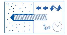
11. Immediately insert the threaded steel anchor / Steel Reinforcement Dowel into the hole using a back and forth twisting motion to ensure complete cover, until it reaches the bottom of the hole. Excess resin will be expelled from the hole evenly around the steel element and there shall be no gaps between the anchor element and the wall of the drilled hole.
