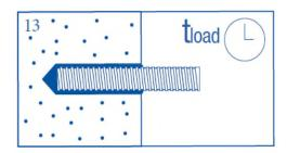
13. Do not disturb the anchor until at least the minimum cure time has elapsed. Refer to the Working and Load timetable to determine the appropriate cure time. Cure time is temperature dependent (>3 hours @40°C)
