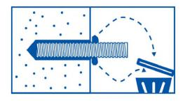
12. Clean any excess resin from around the mouth of the hole using a clean damp cloth or paper towel. Discard correctly. If necessary fit a template in place to ensure the fitted anchors are held in the correct alignment whilst the epoxy sets hard
