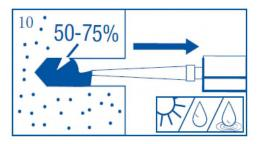
10. Insert the mixing nozzle to the bottom of the hole. Extrude the resin and slowly withdraw the nozzle from the hole. Ensure no air voids are created as the nozzle is withdrawn. Inject resin until the hole is approximately ¾ full and remove the nozzle from the hole. Release the pressure on the cartridge to prevent any further material being extruded accidentally.
