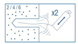
2. Insert an Air Lance to the bottom of the hole and depress the trigger for 2 seconds. The compressed air must be clean – free from water and oil – and at a minimum pressure of 6 bar.
