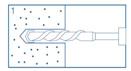
1. Using the SDS Hammer Drill in rotary hammer mode for drilling, with a carbide tipped drill bit of the appropriate size, drill the hole to the required diameter and depth as indicated on the latest **MasterFlow 916 AN** technical data sheet.
