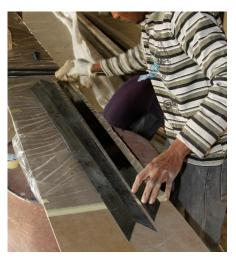
Thoroughly clean the surfaces of the laminate using a white rag and a solvent-based cleaner (Xylene / MEK), in order to remove carbon dust and other contaminants. Cleaning must be repeated until the white rag remains free of black carbon dust and the surface is clean of all contaminants.
