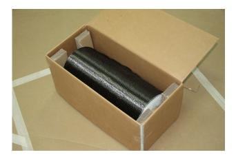
Storage: **MasterBrace FIB** Fabric requires protection against heat, sun and weather. It must be stored on a solid, flat and dry surface, inside a ventilated shelter. If stored in the open, protect with opaque waterproof covers.
