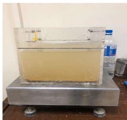
Figure 8 – Deposit of clay on the bottom of glass basin
