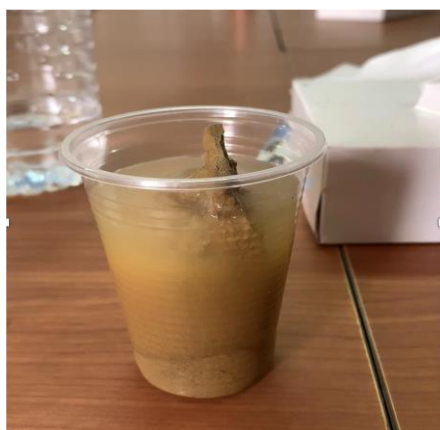
Figure 5 – Clay dissolved when placed in water for one minute
