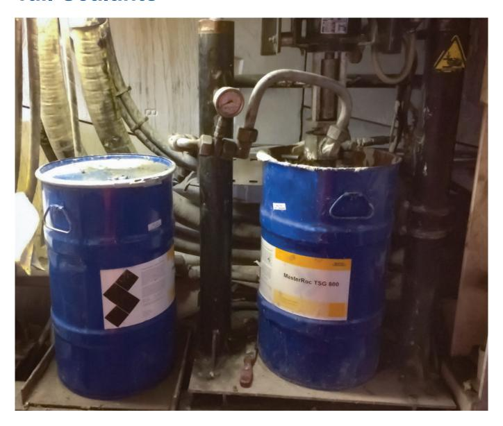
Reliable and cost-efficient sealing of the TBM tail shield is essential for a smooth tunneling operation. Regardless of the soil conditions and the annulus grout type used, the MasterRoc TSG tail sealants effectively prevent not only water but also soil and annulus grout from entering the TBM. Master Builders Solutions offers an inert tail sealant that does not produce any negative side effects for the concrete and the EPDM gaskets.
