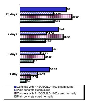
Maximum size of aggregates : 20 mm, Cement content : 350kg/m <sup>3</sup>
