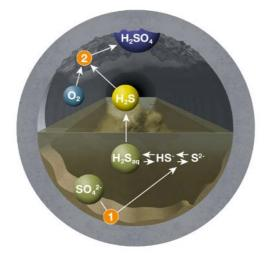
The illustration above represents the different reactions involved in the process of biogenic sulfuric acid corrosion.
