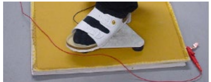
Fig. 5: Testing of surface resistance
