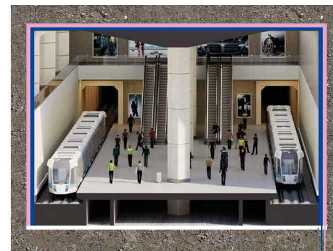
White: MasterSeal 730PA Blue: MasterSeal M 800 / M811 Pink: Protection Board
