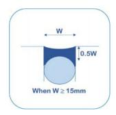
Joint depth is controlled using closed cell backer rod. This also prevents 3-sided adhesion which would be highly detrimental to long term performance of the joint sealant.
