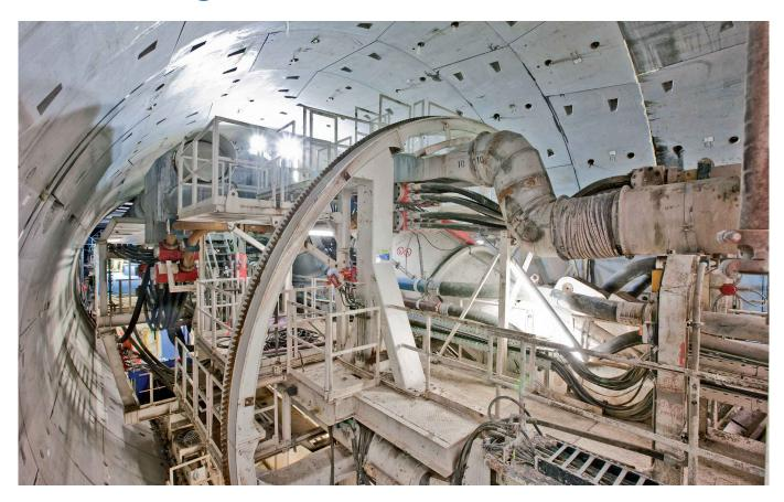
Mechanized tunneling is the safest and quickest way of tunneling especially under difficult geological conditions and in urban areas. The optimum TBM (Tunnel Boring Machine) performance is achieved by combining both mechanical and chemical engineering. Master Builders Solutions provides specialty chemicals for safe and efficient TBM tunneling.
