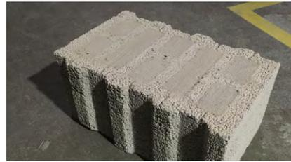
Example of a filled concrete block with insulating foam 35 mW/m<sup>2</sup>K
