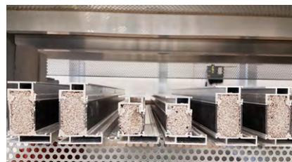
Even small aluminum profiles can be successfully filled and provided with fireproof insulation.
