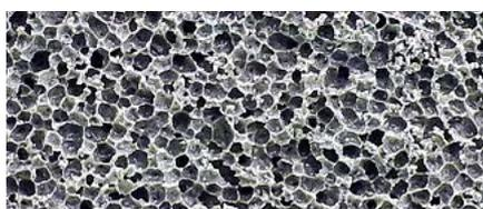
The microstructure of the foam is formed through inorganic polycondensation using alkali-activated aluminosilicates.
