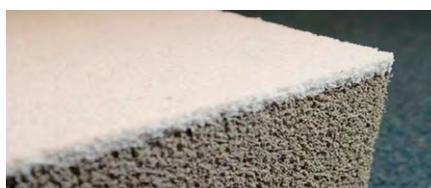
The pores in the microstructure offer excellent sound-proofing and heat retention properties.
