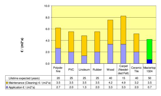
**Graph:** Comparison of life-cycle costs of different flooring systems with PUR based floorings systems of BASF. The life-cycle costs are calculated per 1m<sup>2</sup> and the respective life-time of the flooring system. The application costs of the Mastertop system includes retopping.
