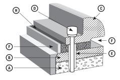
Figure 5 - Typical Epoxy Chock Application
