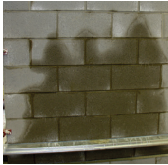
Project # 05-281 - After 72 Hours Back of Reference Wall (no admixture)
